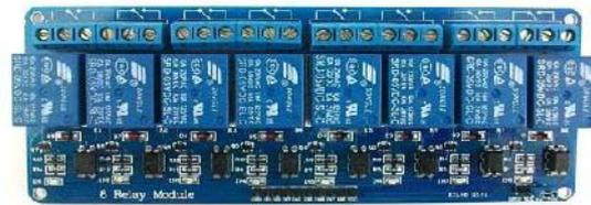
Gambar 4. Relay Board 8 channel
