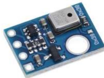
Gambar 3. Sensor AHT10
