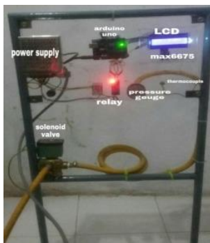
Gambar 2. Pengendali Temperature Control
